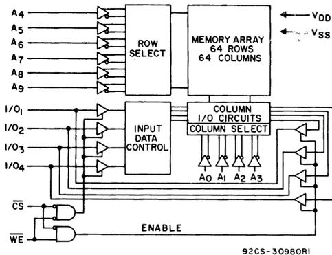
Fig. 1 — Functional block diagram for MWS5114
