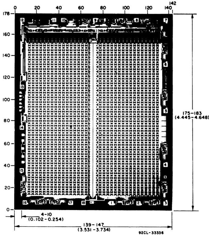
*Dimensions and pad layout for MWS5114H*
