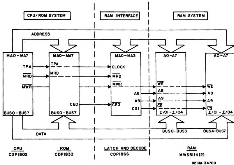
Fig. 5 - MWS5114 (1K x 4) minimum system (1K x 8).
