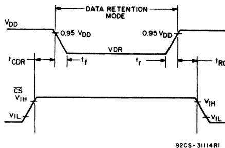
Fig. 4 — Low  $V_{DD}$  data retention timing waveforms.
